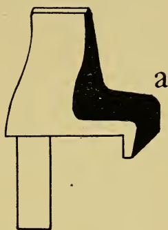
Fig. 19. Hardy made to sit in round hole of anvil.
